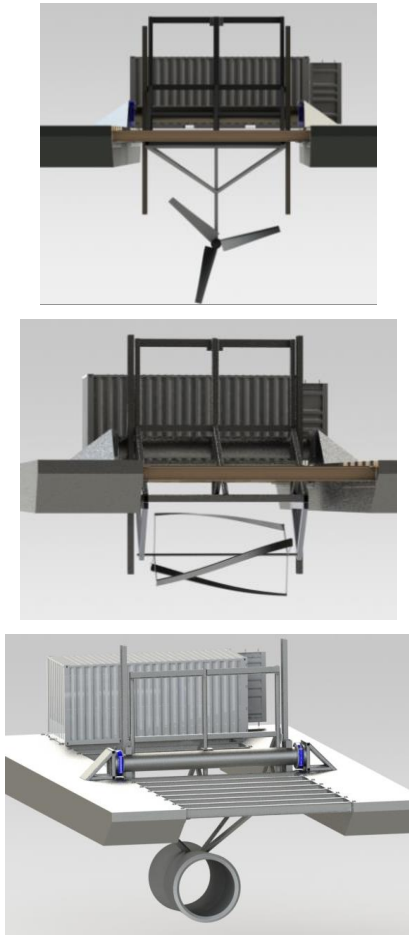
Fig. 9. UNH Tidal Energy Test Platform v2 . Schematic of test platform and MHK turbines: axial (top), cross-flow – horizontal orientation (middle) and ducted (bottom).
