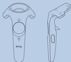
The HTC Vive 6DOF controller. It contains 3 buttons, one analog trigger, and a clickable touchpad for the thumb.
