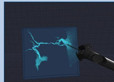
The user could also use a World in Miniature (WIM) style interaction, where a scaled-down model of the particle system can be held and manipulated using the non-dominant hand and the dominant hand can do more precise work, like placing dye pots in areas of interest or probing the flow velocity at ground-trothed locations to quickly assess the model's quality. Any visualizations or interactions occurring on the WIM would also be displayed in the larger particle system in the virtual environment.
