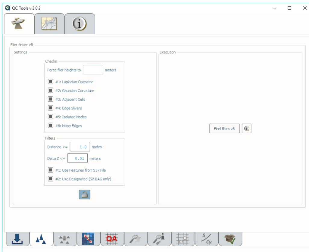
Figure 11 – Screenshot showing the user-interface for Find Fliers v8 in QC Tools. On the left side, the user-modifiable settings (such as which algorithms and filters to apply) are visualized.
