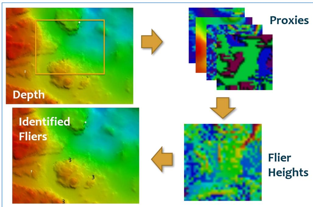
Figure 12 – Workflow adopted to calculate from local proxies and then apply the search height for the Anomaly Detector algorithm.
