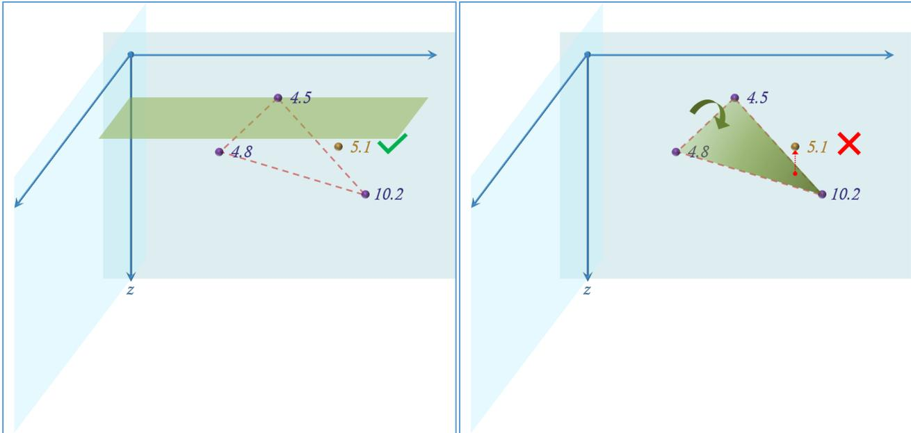
Figure 13 – Example of the application of the traditional triangle test (left pane) and the proposed tilted triangle test (right pane).
