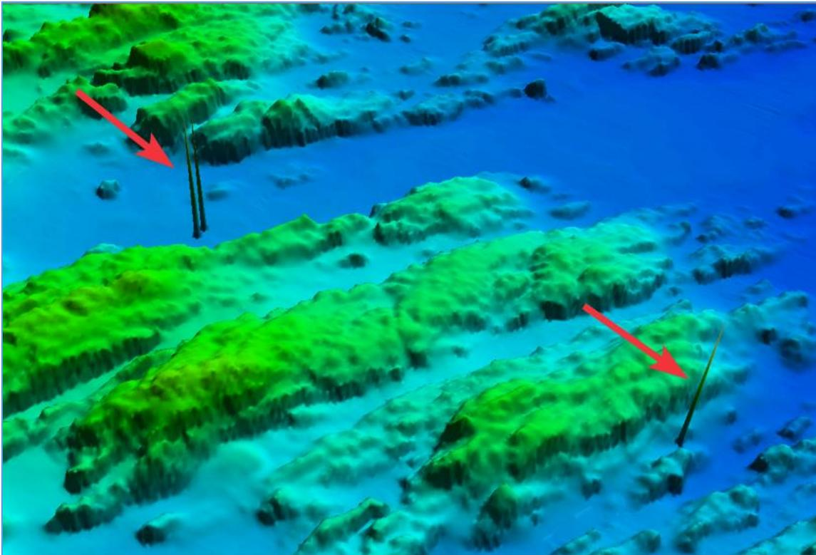
Figure 10 – Examples of anomalous grid data that are not representative of the seafloor (red arrows).
