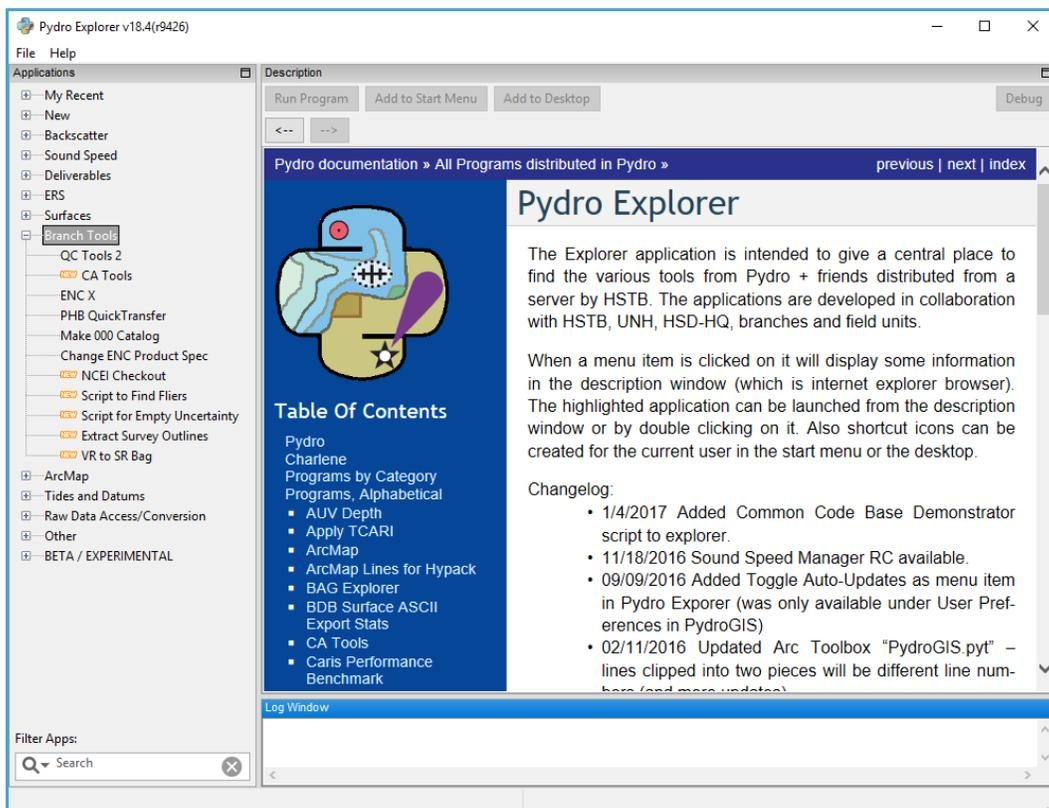
Figure 1 – The Pydro Explorer application helps to access the tools available in Pydro. Each tool is accessible by navigating a tree (on the left side of the application window) where the applications are grouped in themes (e.g., the “Branch Tools” hosts both QC Tools and CA Tools).
