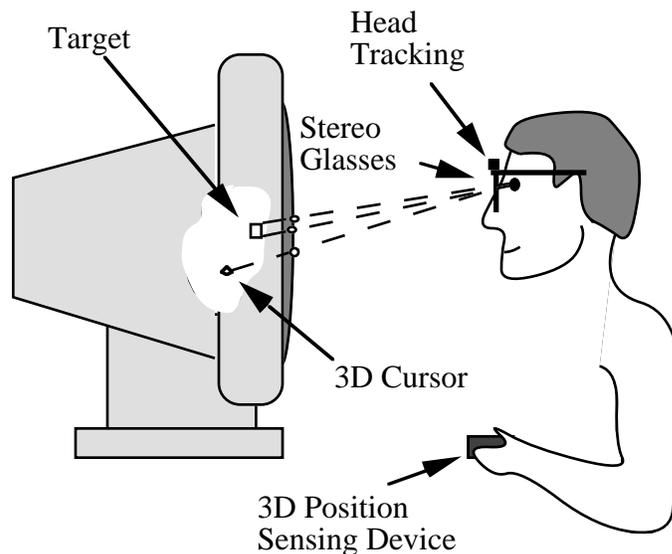
Figure 1. A Fish Tank VR system with 3D positioning using a hand held tracker. The use of a 2D cursor presents a problem if the scene is viewed in stereo.
