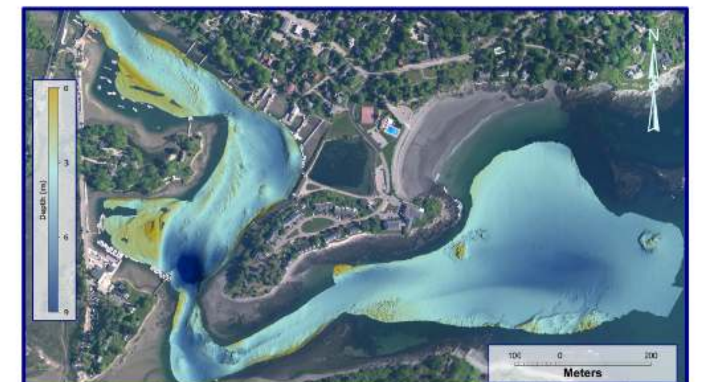
York Harbor - CUBE surface at 0.5-m resolution. UTM 19N, Scale: 1:4,000. Background: 2011 NOAA ortho-rectified mosaic of Maine: Cutts Island to Prouts Neck.
