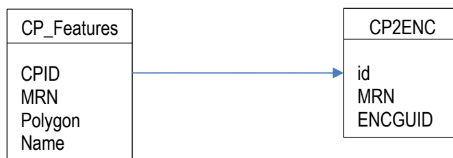
Figure 2. a solution for linking the MRN with each data type, CP_Features is a one-to-one table listing all features in the CP, CP2ENC a one-to-many table to link all the possible changes to ENC data to one CP feature.
